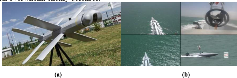
Fig. 8. Typical new drone threats for countering drone radars, (a) Russian Lancet Kamikaze OWA drone [33], (2) Houthi sea drone[34].
